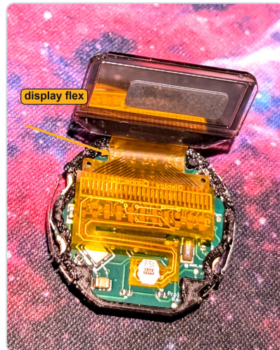
The display up on its flex, before it is folded down into the module.
