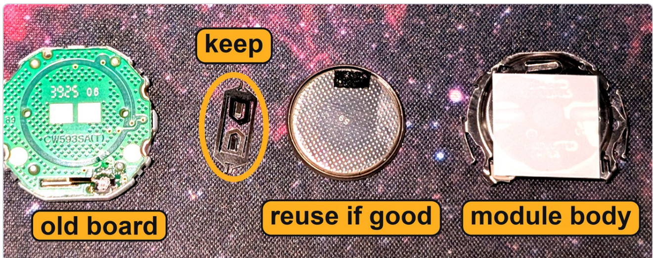
The original module, fully apart. Circled is the battery contact — the second part you keep. The clamp came off in the step above and is not in this frame.
